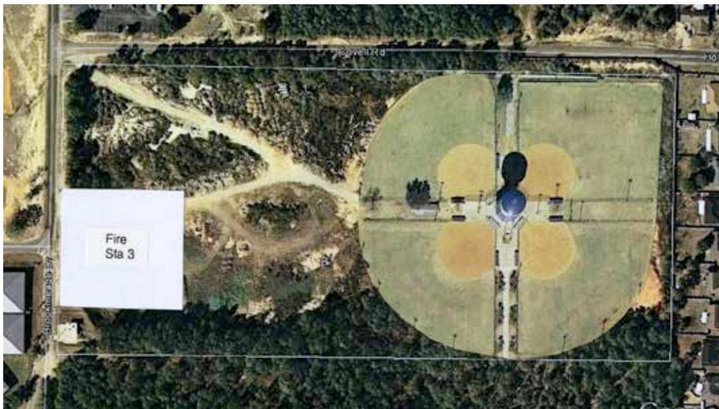
B. Topography: Leveling the playing surface at 200 foot elevation will require considerable sloping on the south side to accommodate the 23' difference ( $200' - 177' = 23'$ ). There are sizeable stormwater retention features on the east and south sides of the Public Safety building. Presumably they must be maintained while providing more stormwater storage on site.
